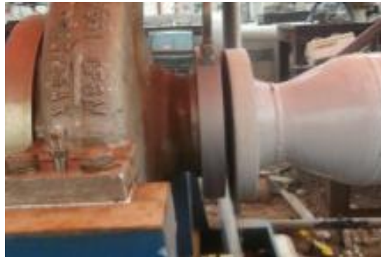
Gambar 3. Kerusakan Flange Pipa (Sumber:Laser Alignment ReportCGS)
