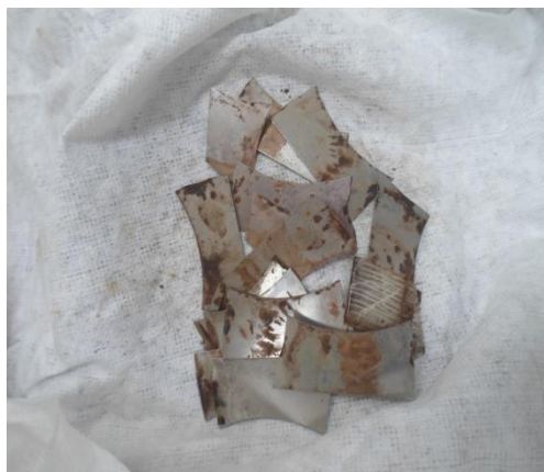
Gambar 3. Kerusakan Flange Pipa (Sumber:Laser Alignment ReportCGS)
